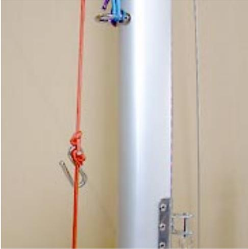
The topping lift is adjusted so that, when hooking up the pole, it will set approximately parallel to the water. It will then be readjusted for the conditions after the spinnaker is set. When the pole is not in use, the hook will lie about 10" below the ring fitting.
