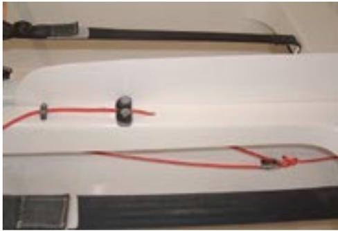
Once through the cap, the end is attached to a single block. A second red line, which is dead-ended under the back of the cap, is then passed through the block and back up through the cap to a CAM cleat. The reason for this type of cleat, as opposed to the Clamcleat is that the rope will run free, unattended, once released and the crew does not have to hold it to keep it from jamming.
