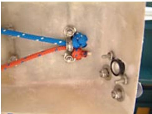
This picture shows the vang (blue), and the c/b downhaul (red), sharing the deckstrap under the cap. The angle of the rope from the tongue of the board to the exit box is fine for sailing but it does not hold the tip of the board firmly in the box. When through sailing, wrap the line once around the tongue to be able to pull the board ALL THE WAY UP.
