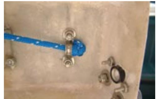
A close up of the bottom block and its attachment is shown below with the first and second parts coming off the shackle and the third part off the block.
