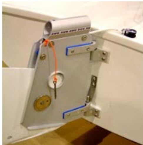
shown. It may be convenient to place the blade in the "up" position and secure there by tightening the black locknut which we have placed on the port side of the rudder head. This may be reversed if the starboard side is found more convenient. Use
