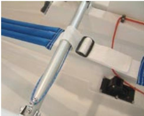
Above, the straps held in place. Below, the simple bridle system. The bridle is attached to a shackle at each end and the shackle is attached to the existing eyestay. The height of the straps is adjusted
