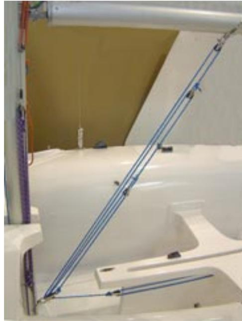
The boom should still be held up by the main halyard, or sail. Attach the single block with the shackle (the first part) to the boom as above. This will leave a single piece of line, with a block attached (the third part) coming off the bottom block attached to the mast. You will find a blue line in the boat on the port side of the board box with its end attached to nothing
