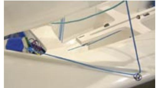
end is rigged, typically, outside the jib, through the guy hook, then to the spinnaker head in the bag.
