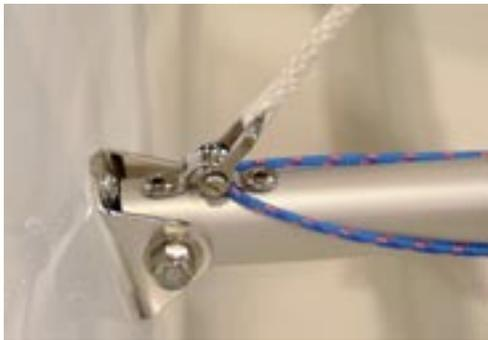
by the yellow hiking strap adjuster rope. One end is tied off at the deck strap. The other goes through the loop in the straps, back through the eyestay then is tied off on itself in a bowline. Adjust this end of the line for height because the other has the topping lift shockchord retractor attached to it. See bottom picture.
