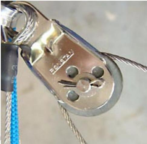
jumping the sheave. If you ever remove the sheave be sure to put back the washer. Also, examine the shroud and trapeze wire attachment. They are on the same tang as shown. A shrink wrap tube is then
