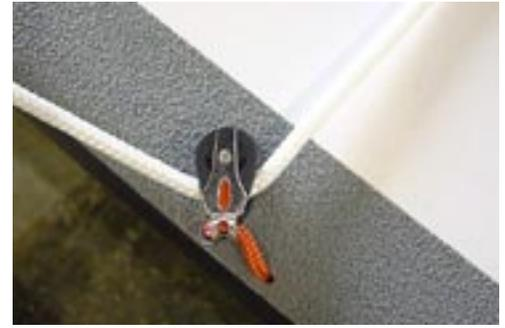
crews prefer to use a continuous sheet with the two ends tied off at the clews. The only disadvantage is that there is always a sheet across the centre of the boat. The sheet is shipped as a single line allowing for this. It may be cut to provide two individual sheets.
