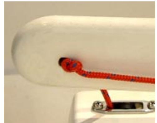
The line is knotted on the other side of the board where it now becomes the uphaul. It then passes down through an exit box in the cap of the centreboard case.
