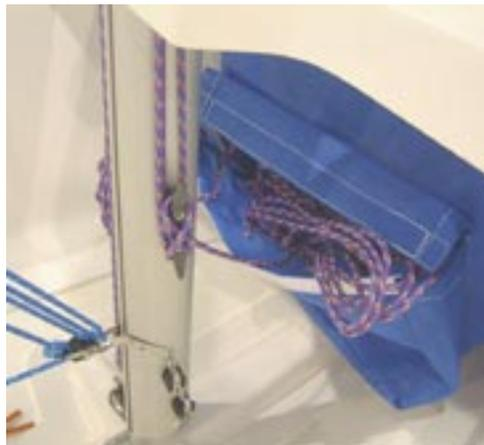
and back up through the loop. Tension firmly, tie off on the cleat and stow the tail in the pocket of the spinnaker bag
