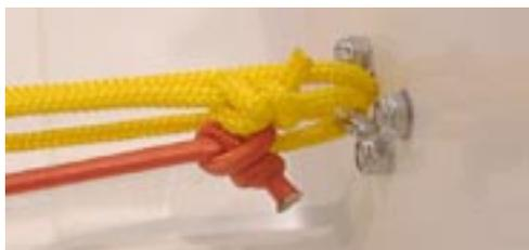
The straps are kept tensioned and off the floor by a shockchord loop that runs from an eye on the transom down around the adjustment rope assembly and back up to the eye. Extra shockchord is provided so that adjustments can be made.
