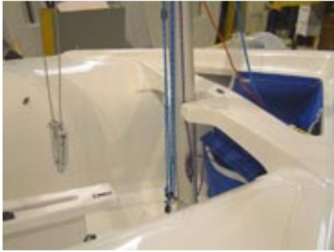
Position the mast in the partner and attach the forestay to the centre pin in the bow fitting. The mast can now
