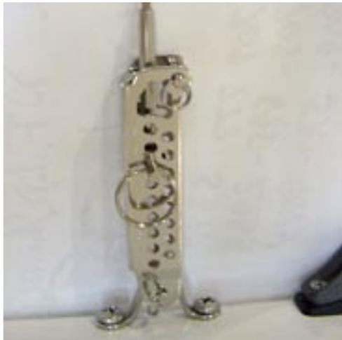
a second pin in the top of the chainplate which must be removed to allow the shroud to pass. Replace this after pinning the shroud as it is a safety device if the main pin happens to come loose (It happens!)
