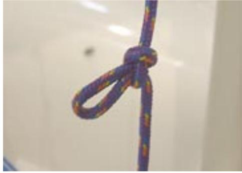
as shown in the following picture. Some Club 420s use a stainless ring knotted into the halyard but this is as effective, particularly if you put sun-screen in the end of loop. Pass the halyard around the cleat
