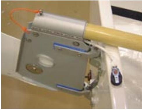
Fit tiller into rudder head and pass the cotter pin through the tiller, making sure that it also goes through the rudder head on the underside.
