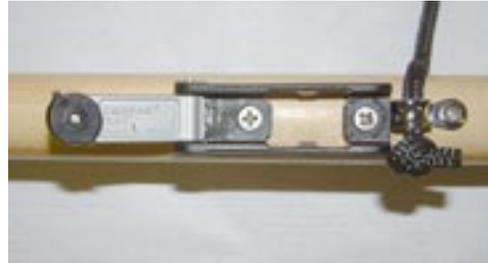
to check the operation, gently pry the cleat open with a flat screwdriver and observe the position of the cam. Also check that the set screw is firmly tightened. - the cam must be held from turning when the screw is tightened. Do not over tighten or you will strip it! Snap back into place.
