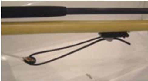
Pass the line from the cleat through the block and take it back to the cleat. Once the boat is in the water, loosen the lock nut on the rudder head, pull the line firmly tight and
