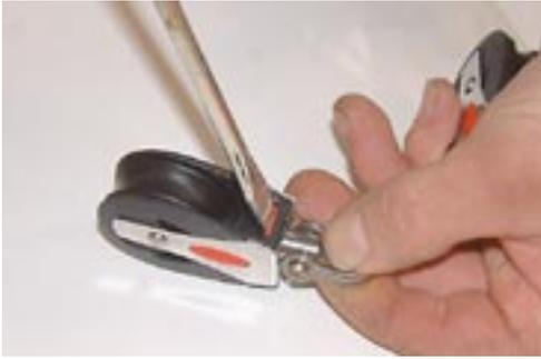
Make sure that the blocks are aligned fore and aft then lock them in that position. They usually leave the factory fully swivelling but there is a small, flat, red locking tab which can be pushed across the block to lock it on either 90 degree axis.
