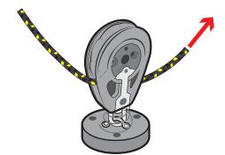
b) • Next, thread the mainsheet through the block in the middle of the boom, leading it towards the back of the boat.
