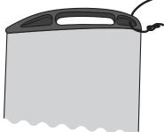
b) • Tie the daggerboard retaining clip on to the other end of the daggerboard retaining elastic using a knot on a knot.
