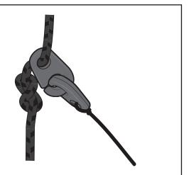
The Inglefield Clips stop the halyard flopping around when the mainsail is hoisted. To lower the mainsail, release the Kicker, outhaul and downhaul and unclip the two clips, pull the halyard out of the cleat at the top of the mast, and pull the mainsail down.
